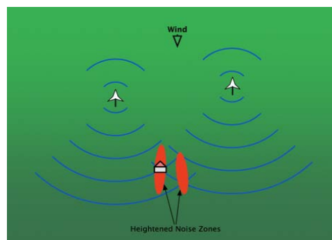
Figure 10: Noise from 2 turbines creating Heightened Noise Zones
